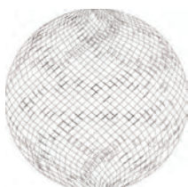
Orbitor 4 nozzle spray pattern
