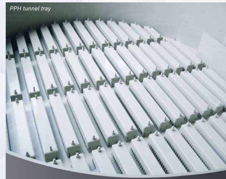
Installation of tunnel caps at a tunnel tray
