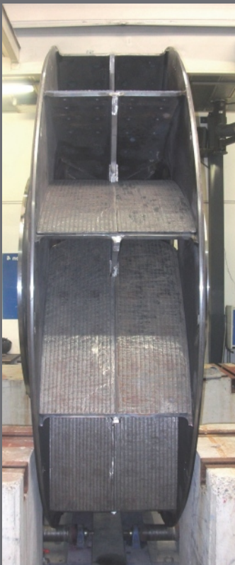
Impeller with welded composite armour plate.
