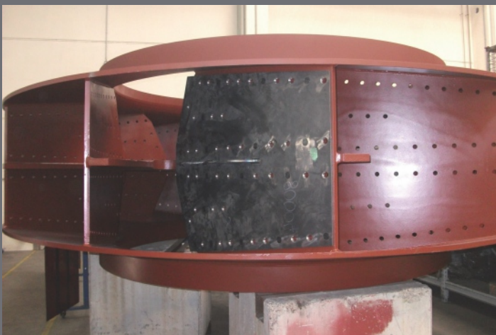
Impeller with screw-on wear protection.
