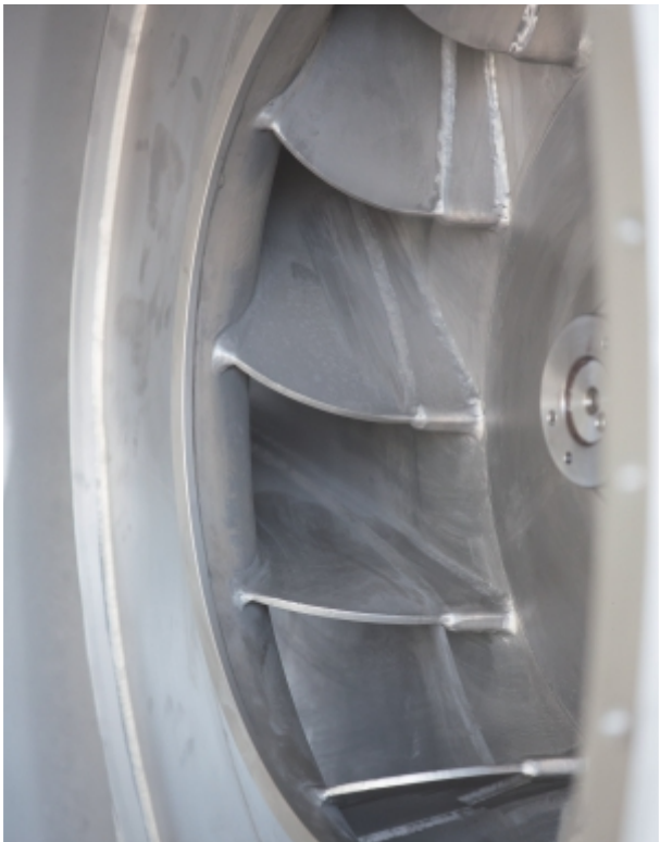
Centrifugal Impeller made of stainless steel
