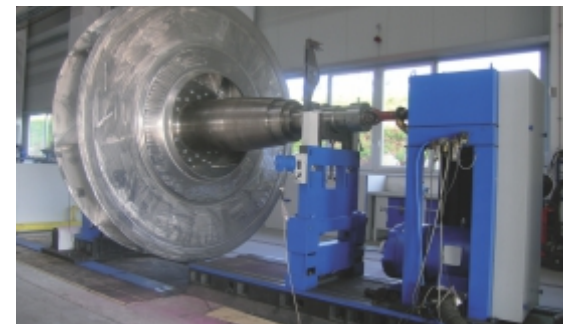
Centrifugal rotor on TLT-Turbo balancing machine
