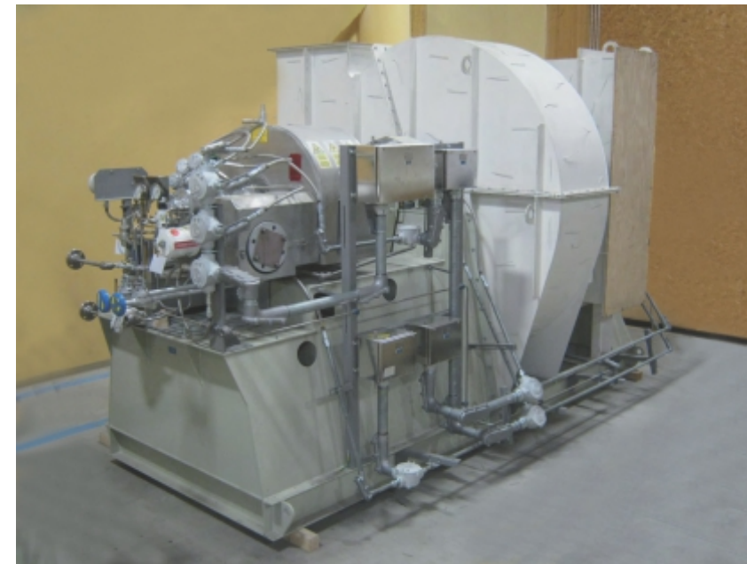
Centrifugal fan with steam turbine for a petrochemical application
