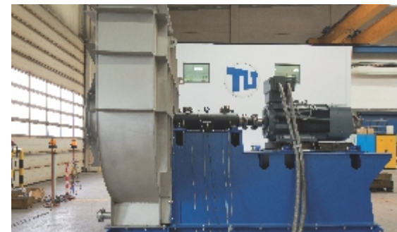
Centrifugal fan with electric drive during workshop test
