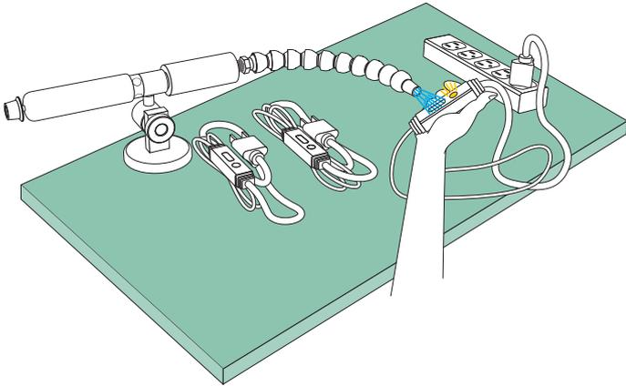
**The Problem:** A manufacturer of electrical heat tapes had a problem testing thermostats for accuracy. The heat tape is supposed to switch on when the outdoor temperature dips below 40°F to prevent pipes from freezing or ice from building up on a roof's edge. The liquid-tight thermostat of every tape had to be dipped into a bowl of ice water (thermometer checked at 36°F (2°C)) to make sure the indicator light
