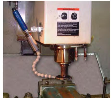
**The Adjustable Spot Cooler replaces flood coolant and eliminates hours of cleanup on a cast iron machining operation.**
