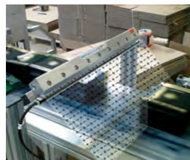
The Model 112118 18" (457mm) Gen4 Super Ion Air Knife System eliminates dust from body care products prior to sealing the boxes in cellophane.
