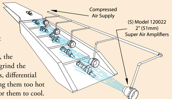
**The Solution:** They installed **(5) Model 120022 2" (51mm) Super Air Amplifiers** over the shake-out conveyor. The high output airflow from each Super Air Amplifier rapidly cooled the parts without shocking them (no cracks or imperfections from cooling too rapidly). **When the part reached the end of the conveyor, the operator could proceed immediately.** The backlog was completely eliminated.
