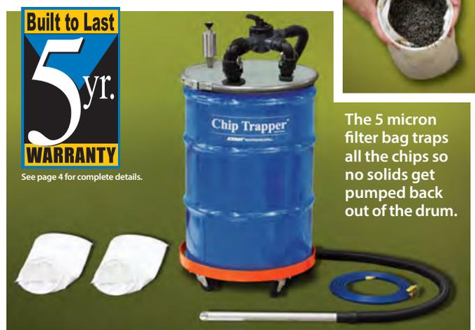
The Chip Trapper includes the pump assembly with directional flow valve, a 30, 55 or 110 gallon drum, 10' (3m) chemical resistant hose, 20' (6.1m) compressed air hose, aluminum chip wand, (2) reusable 5 micron filter bags and drum dolly.
