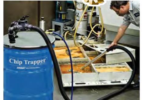
Chips can accumulate in the sump, restricting coolant flow.
