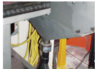
Metal parts are conveyed with the Model 150200 2" (51mm) Heavy Duty Line Vac as they drop off the edge of the conveyor.
