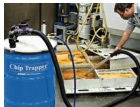
Chips can accumulate in the sump, restricting coolant flow.
