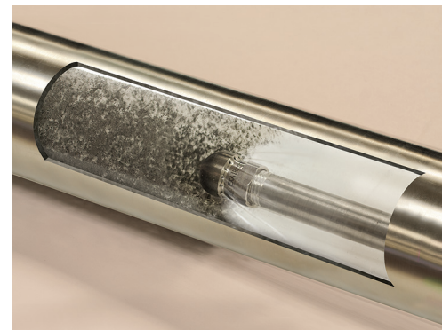
A Back Blow Air Nozzle cleans chips and coolant from inside a machined pipe.
