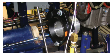
A Model 120024 4" (102mm) Super Air Amplifier cools an engine during dynamometer testing.
